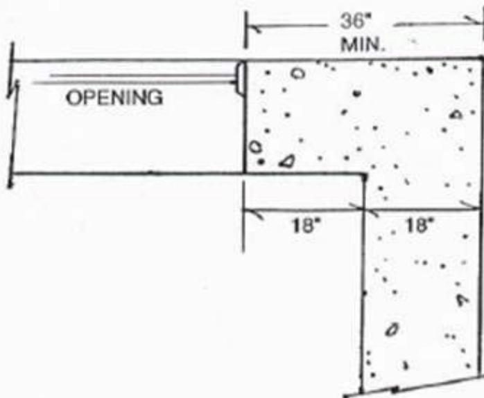
THE MINIMUM DISTANCE MEASURED FROM THE EDGE OF ANY OPENING TO THE NEAREST CORNER, PLUS THE ADJOINING WALL THICKNESS SHALL NOT BE LESS THAN 36 INCHES
